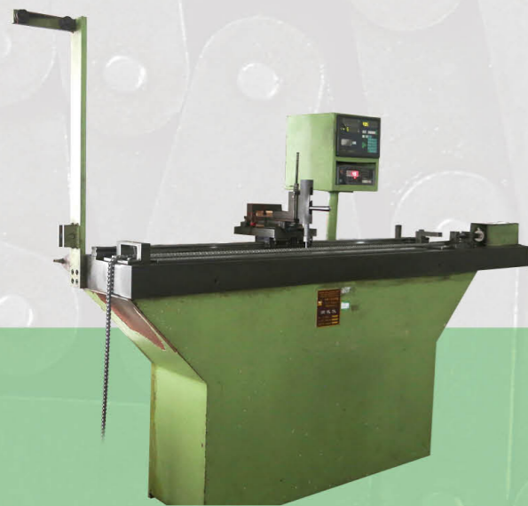
链长仪 Chain length inspection
